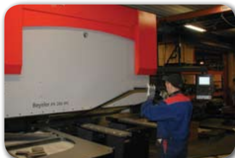
Forming is carried out in CNC automated edge press machines.
