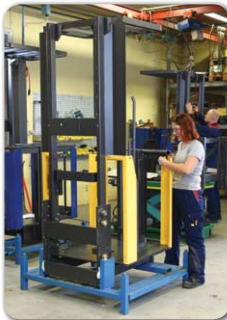
We perform the assembly of large and small components. We also have a specialised section for testing/ cleaning, together with the assembly of hydraulic and fuel tanks.
